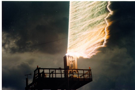
Figure 1: A rocket-triggered strike at Camp Blanding, Florida [ source : lightning.ece.ufl.edu].
