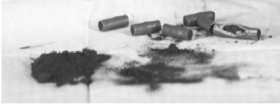
Figure 3: Spent Fuel after voloxidation. It can be seen that chopped fuel rods have been reduced to powder due to voloxidation process and that fuel rods have been ruptured. 25
