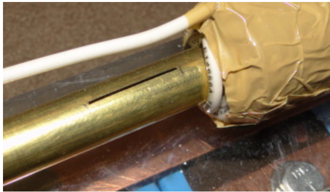
Figure 7: Slot in brass barrel to minimize eddy current generation.
