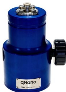
Figure 1.1: Photograph of the qNano instrument. A USB connection provides electronic control from, and data logging to, a laptop or PC. The side knob provides mechanical control of the membrane stretching distance by adjusting the width of the jaws.
